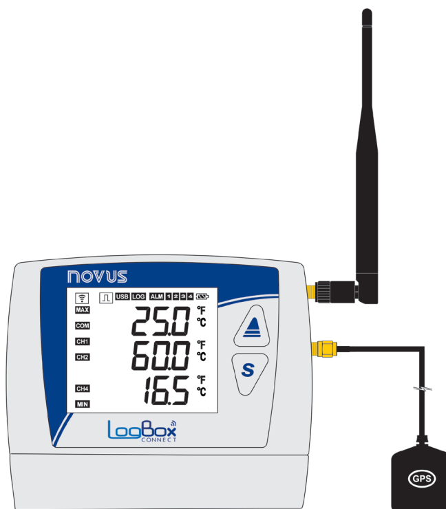
Fig. 45 – Cellular and GPS Interface
