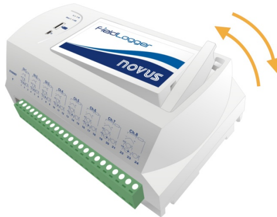
Fig. 08 – Attaching and detaching FieldLogger front cover
