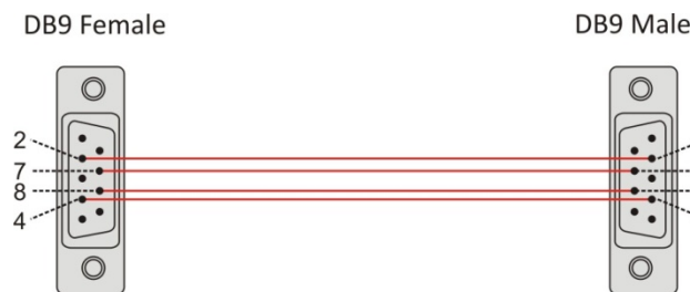
Fig. 26 – Building an extension cable
